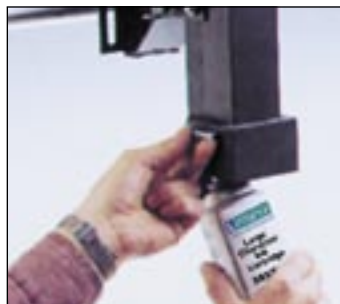
Self-contained pressurized ink container provides fast, clean ink changes.
