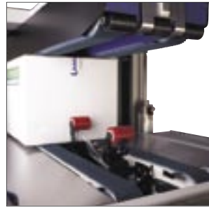
Top and bottom belts provides the most reliable drive style
