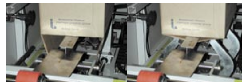
Folds all four bottom flaps pneumatically in the stationary position.
